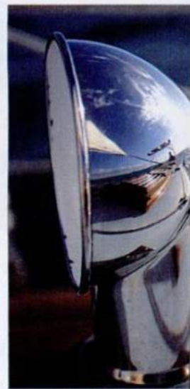
A period skylight and chrome-plated dorade vents identify the early Alajuuela as a traditionalist's boat.
